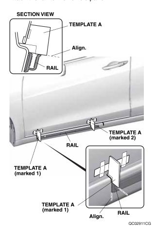
14. Make sure that the rail is aligned with each template, then carefully remove each adhesive backing.
