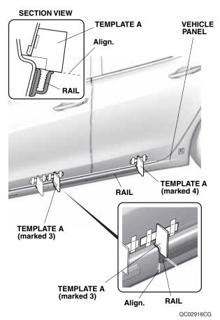
20. Make sure that the rail is aligned with each template, then carefully remove each adhesive backing.
