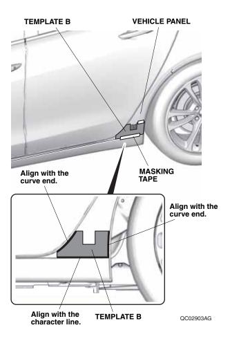
3. Using a felt-tip pen, mark the vehicle panel as shown. Remove template B. Be careful not to damage the template. It will be used to mark the right side of the vehicle.
