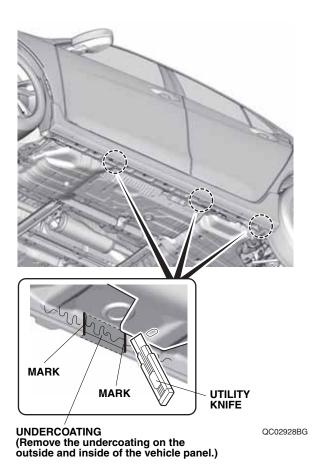
41. Apply touch-up paint to the area where you removed the undercoating, and allow it to dry thoroughly.
