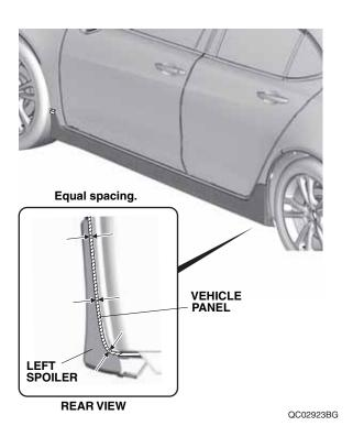
27. Lightly tap the spoiler to remove any gap between the spoiler and the left front fenderwell.
