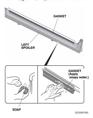
25. Secure the hook on the spoiler to the bracket and align the gasket on the spoiler with the rails. Insert the rear part of the gasket into the rail first, then work forward. Move the spoiler up and down gently to make sure that the gasket is installed securely to the rails.
